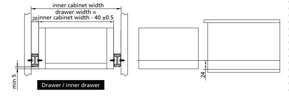
The bottom of drawer slides The center of drawer slides must be 24mm must be 5mm above the above the bottom of cabinet. bottom of drawer to ensure correct function.
