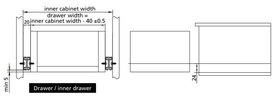
must be 5mm above the bottom of drawer to ensure correct function.
