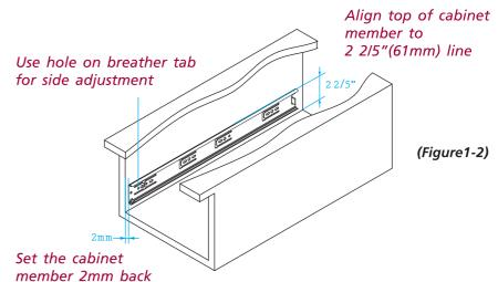
Fix the slides through the most flexible holes on breather tab for best slide performance. Leave the screw loose for final adjustment.
