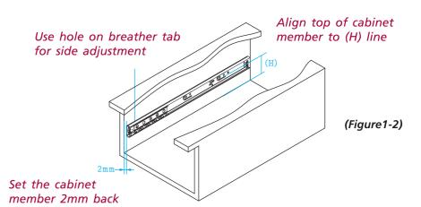
Fix the slides through the most flexible holes on breather tab for best slide performance. Leave the screw loose for final adjustment. Move the slides back and forth, and make sure no screw is bound.
