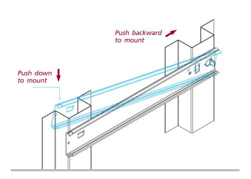
For the ease of installation, suggest mounting the slides from the bottom to the top.
