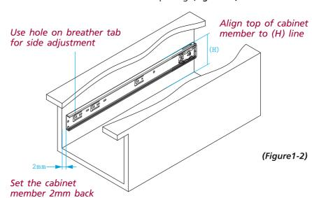
Fix the slides through the most flexible holes on breather tab for best slide performance. Leave the screw loose for final adjustment. Move the
